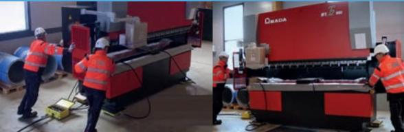
Air skates are robust, low profile, high capacity load-moving modules used in sets of four or six to enable large or heavy objects to be moved with ease.
