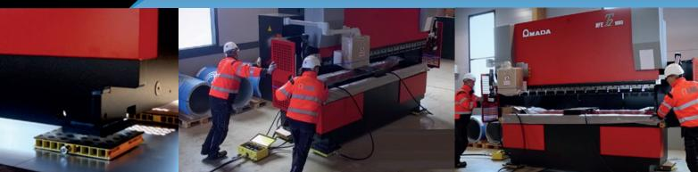
Air skates are robust, low profile, high capacity load-moving modules used in sets of four or six to enable large or heavy objects to be moved with ease.
