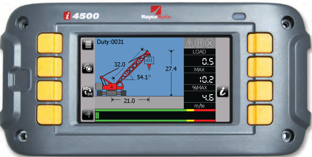
i 4500 • 4.3" display • 480x272 pixels resolution screen
